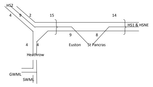
As may be seen in the diagram above, the key to efficient path utilisation on a HSR network as proposed here is the use of delta junctions and the creation of cross-Heathrow and cross-London linkages, including between HS1 and HS2.
